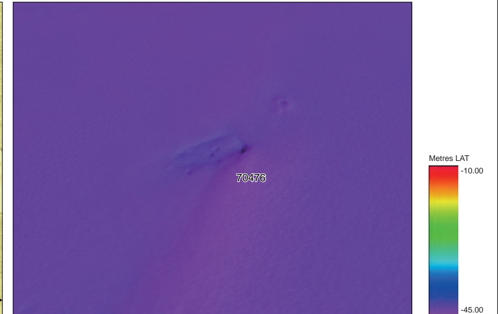
MBES grid image, x 1 vertical exaggeration, looking north
